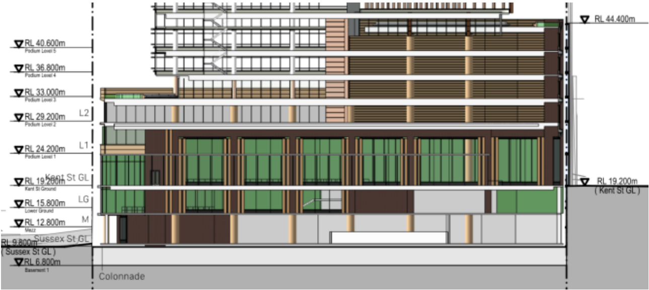
Figure 4 - Architectural East-West section
